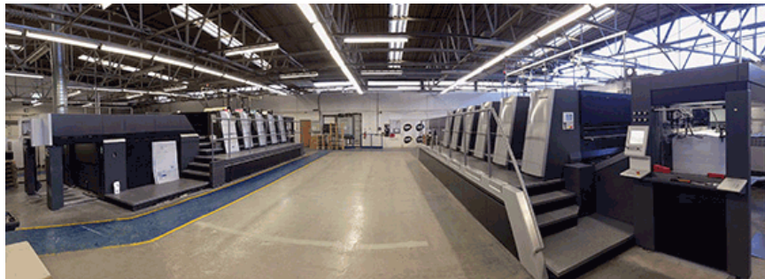
ESP Colour's pressroom with the Heidelberg XL105 and XL106 machines, claimed as the world's most productive presses. Between them they print 155 million impressions per year.
